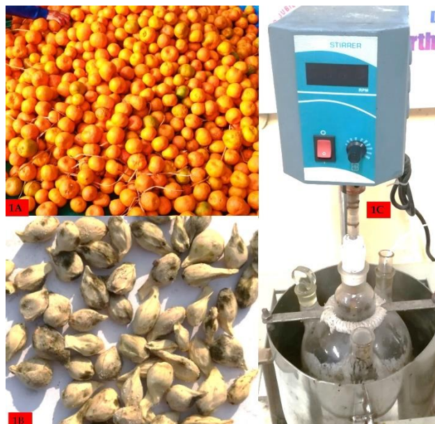
Figure 1A. The fresh and ripen Orange ( Citrus x aurantium L.) fruits collected from local vendors for extraction of seed oil; 1B. The sun dried Orange seeds from ripen orange used as raw material for non-edible biodiesel production; 1C. Biodiesel reactor used for extraction of orange seed oil for biodiesel processing.
